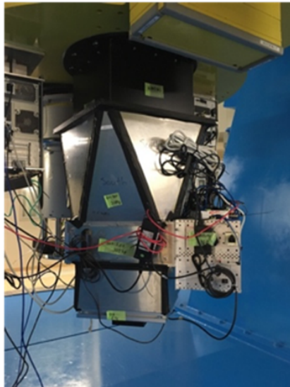
Fig. 1. WFGS2 attached to the Cassegrain focus of Nayuta telescope.
