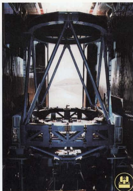
Top ring being installed at shop erection of the SUBARU Telescope
