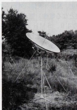
Fig.1 Antennas we built at Nishi-Harima Astronomical Observatory. a) half-wave dipole, b) 5 element Yagi, c) parabolicreflector antenna(1.2m in diameter), d) conical log-spiral antenna.
