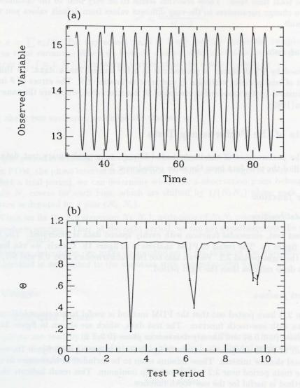
Fig. 1. A test result of PDM library. (a) A test data with sinusoidal function and (b) the result of PDM library are shown.
