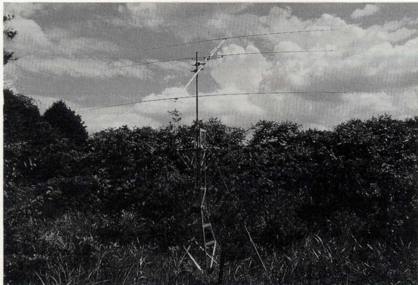
Fig. 2. One of the three-element Yagis used for interferometer observations.
