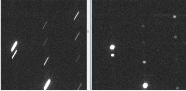
**Fig. 5.** The image obtained with the slit use for observation (left panel) and the image of the slit for test observation (right panel) are presented. In the test observation slit, the image looks like a pinhole image.
